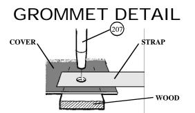
Position the blue strap on the cover. With the hole punch provided (item #207), punch a hole through the strapping and the cover. Ensure that the hole in strapping is at least 1 1/2" from the end of the strap and that the hole in the cover is at least 1 1/2" from the end of the cover. Use a piece of wood to avoid damaging the hole punch.
