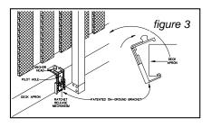
**STEP 5** FOR ADJUSTABLE BRACKET ONLY, INSERT THE BLACK SPACER BLOCKS INTO THE BRACKETS (**DOES NOT APPLY TO ONE PIECE METAL BRACKET.**) ONCE THE BRACKETS ARE FASTENED TO THE DECK. <u>Please Note</u>: See *Figures* 4, 5, and 6 for proper placement of the Spacer Blocks for Kayak On-Ground pools vs. all other brands. All Brackets <u>MUST</u> be used with the Spacer Blocks or the LOOP-LOC warranty will be void.
